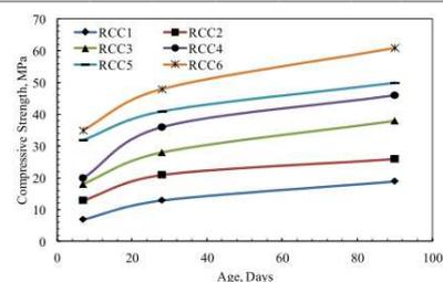
**Figure1. Compressive strength gain as a function of time after casting**
