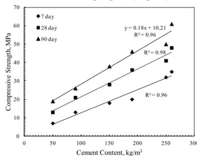
**Figure 2 Influence of cement content on compressive strength for different curing ages**
