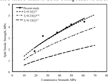
**Figure 6 Relationship between compressive strength and split tensile strength**
