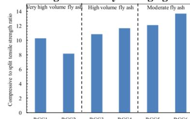
**Figure 5 Compressive to split tensile strength ratios for RCCs investigated at 90 day curing Age**
