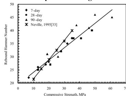
Figure 8 Relationship between rebound hammer number and compressive strength
