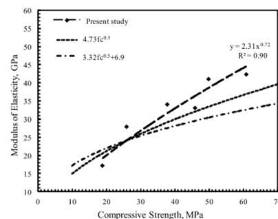
Figure 7 Relationship between modulus of elasticity and compressive strength
