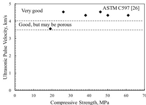
**Figure 9 Relationship between compressive strength and ultrasonic pulse velocity**
