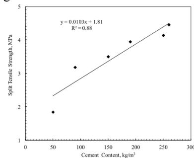
**Figure 4 Influence of cement content on splitting tensile strength at 90 day curing age**
