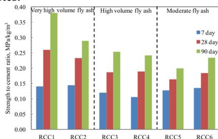
**Figure 3 Strength to cement ratios for RCCs investigated at different test ages**
