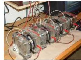
**Fig.-2. Concrete specimens under RCPT**
