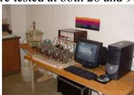
**Fig.-1. Running RCPT on 4 concrete specimens**
