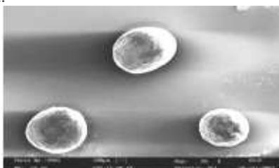
**Fig 1. SEM photomicrograph of calcium alginate beads**
