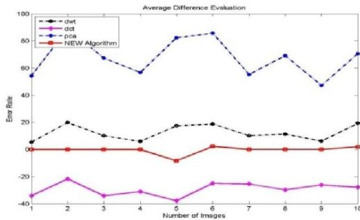
Figure 4.3 has shown the quantized analysis of the Average Difference of different images using fusion by DWT transform (Black Color), fusion by DCT transform (Magenta Color), fusion by PCA transform (Blue Color), fusion by Proposed Approach (Red Color).
