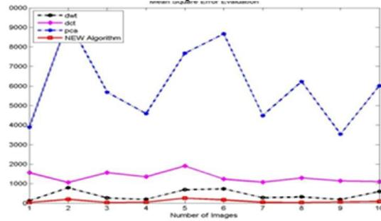
**Figure 4.1 MSE of DWT, DCT, PCA& Proposed Approach for different images**
