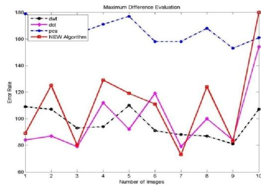
Graph 4.6 MD of DWT, DCT, PCA & Proposed Approach for different images
