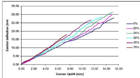
Figure 3.1.6 Central Deflection Vs Corner Uplift at Corner B
