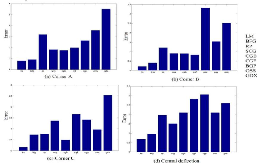
**Fig 3.1.6 Comparison graph for different algorithm in Slabs with two ends discontinuous and other ends continuous**
