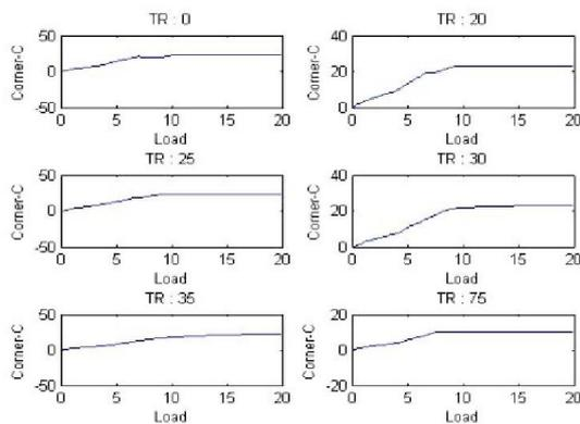
**Fig 3.1.9 (c) Corner uplift in Slabs with two ends discontinuous and other ends continuous Corner C**
