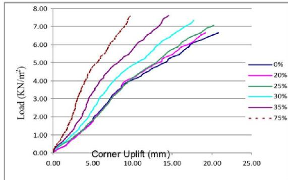
Figure 3.1.3 Load Vs Corner Uplift At Corner C
