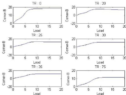
**Fig 3.1.9(b) Corner uplift in Slabs with two ends discontinuous and other ends continuous Corner B**
