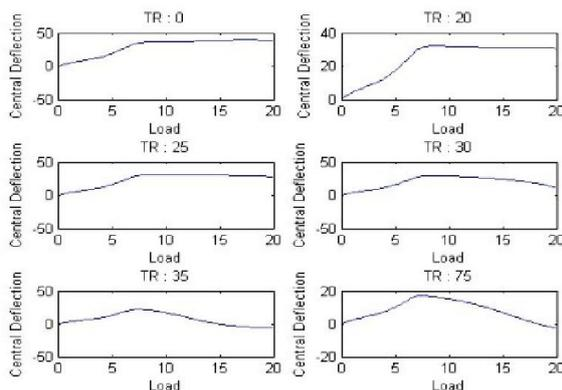
**Fig 3.1.9(d) Central deflection in Slabs with two ends discontinuous and other ends continuous**
