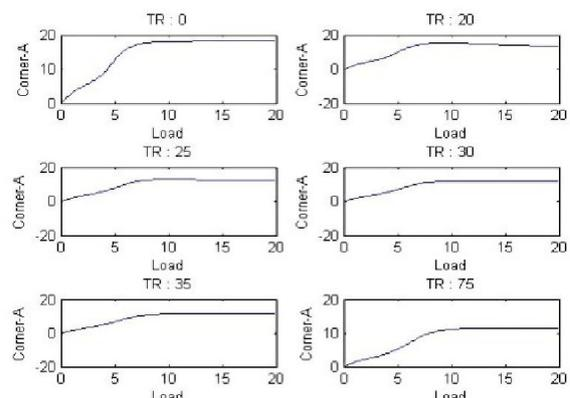
Fig 3.1.9 (a) Corner uplift in Slabs with two ends discontinuous and other ends continuous Corner A
