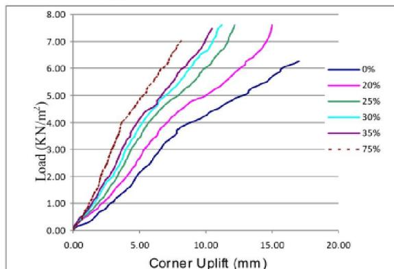
Figure 3.1.1 Load Vs Corner Uplift at Corner A
