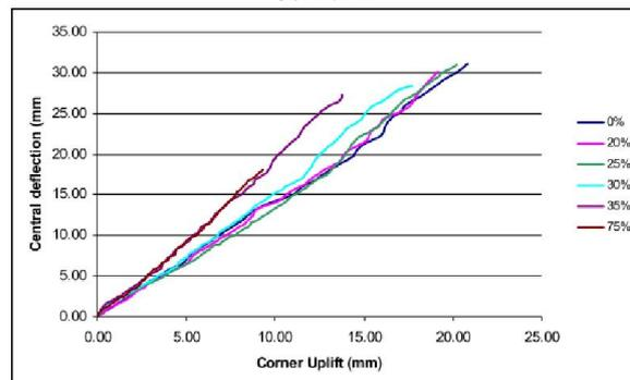
Figure 3.1.7 Central Deflection Vs Corner Uplift at Corner C
