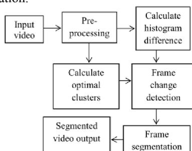
**Figure 1: Basic Block Diagram of Video Segmentation**
