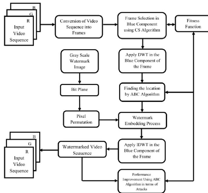
Figure1. Structural Design of Hybrid Video Watermarking
