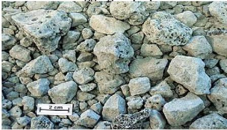
**Picture2: Granulated blast furnace slag (GBS)**
