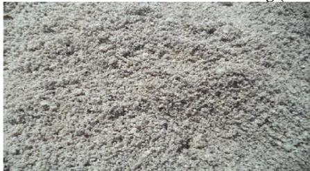
**Picture 3: Electric arc furnace slag in hot condition**
