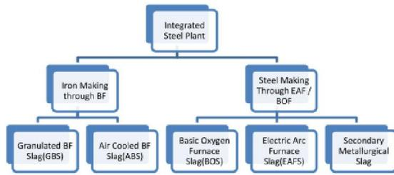
The slag generated during iron making from BF and Steel making from BOF/EAF are classified as BF Slag and Steel slag:
