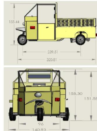
Fig. 5 (a) and (b): Side and Front views of tricycle with dimensions in cm (CAD)
