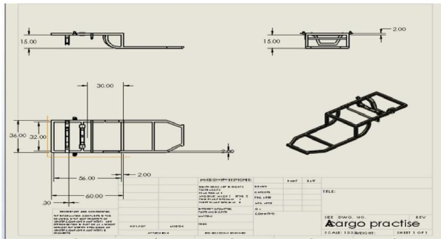
**Fig. 1: Chassis frame (Top, side, back, and isometric) with Computer Aided Design (CAD)**
