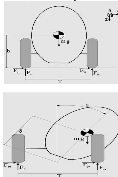
Fig. 4 (a) and (b): Forces acting on a narrow vehicle
