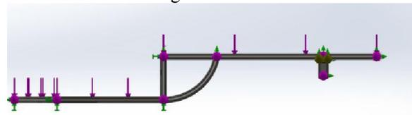
**Fig. 3: Major loads acting on the chassis frame**
