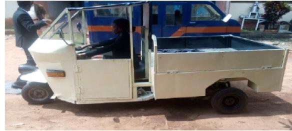
Fig. 6: Side view of the completed load-bearing tricycle.
