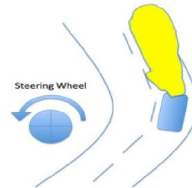
Fig. 2 Turning of head lamps with respect to steering wheel
