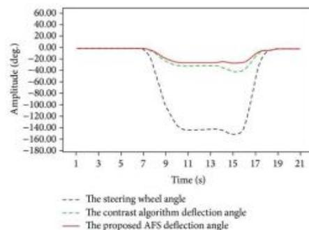
**Fig. 3 Head lamps deflection angle and steering angle**
