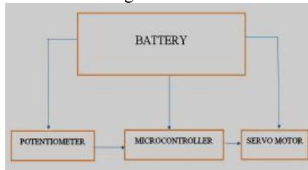
**Fig. 4 Block diagram of adaptive lighting system.**
