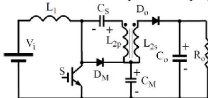
**Fig. 3. Modified SEPIC converter with magnetic coupling.**
