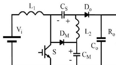
**Fig. 1. Modified SEPIC converter without magnetic coupling.**
