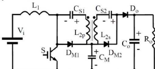
**Fig. 4. Proposed converter - Modified SEPIC converter with magnetic coupling and output diode voltage clamping.**
