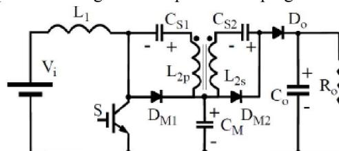
**Fig. 2. Proposed converter - Modified SEPIC converter with magnetic coupling and output diode voltage clamping.**
