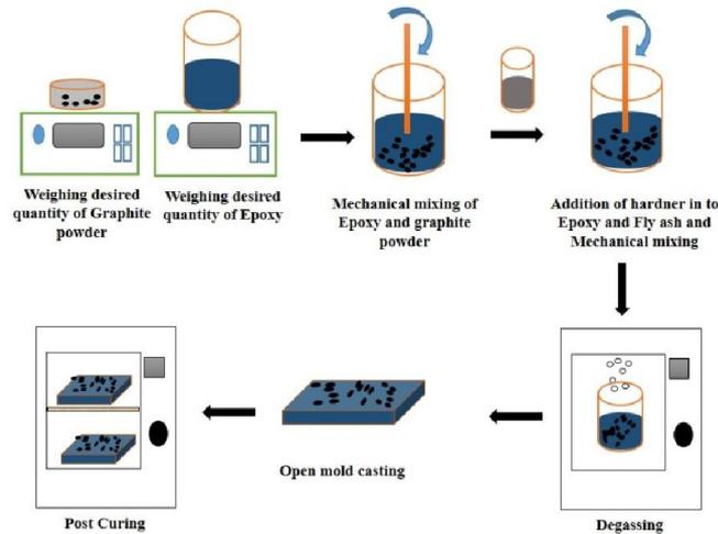
Fig. 2. Schematic for preparation of Epoxy/Graphite composites
