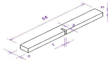
Fig. 5. Specimen Dimensions for Fracture Toughness Test
