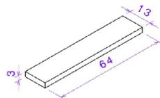
Fig. 3. Specimen dimensions for Charpy Test
