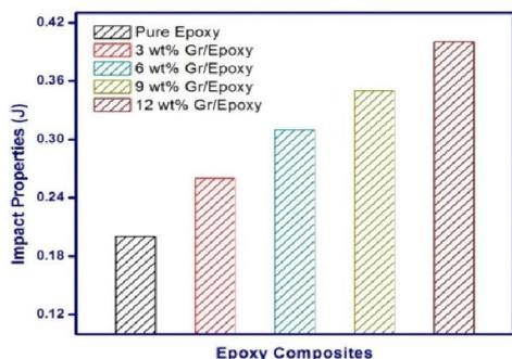
**Fig.7. Impact Properties of Epoxy/graphite composites**
