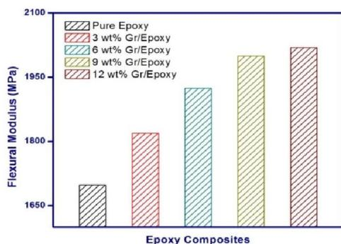
**Fig.9. Flexural Modulus of Epoxy/graphite composites**
