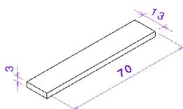
Fig. 4. Specimen Dimensions for Three Point Test
