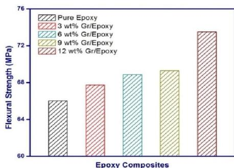
**Fig. 8. Flexural Strength of Epoxy/graphite composites**
