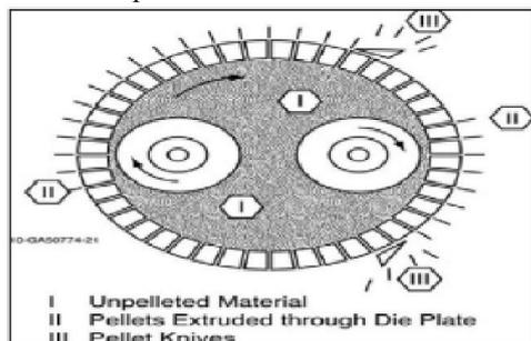
**Fig.1 schematic of pellet mill<sup>24</sup>**
