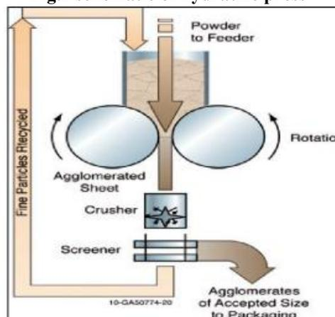
**Fig.3 schematic of roller press<sup>24</sup>**
