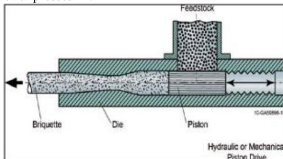
**Fig.2 schematic of hydraulic press<sup>24</sup>**
