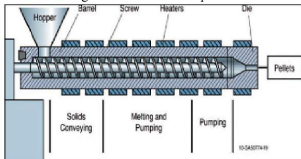
Fig.4 schematic of screw extruder<sup>24</sup>
