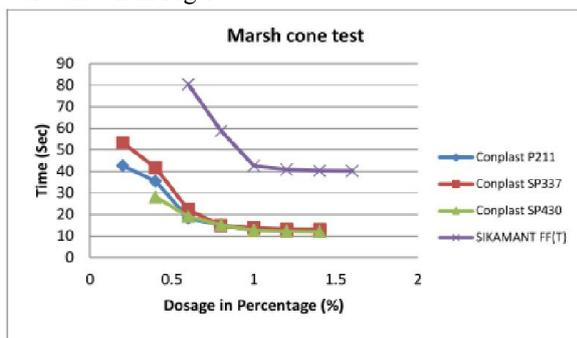
**Fig 1. Optimum Dosage of Super plasticizer using Marsh cone test**
