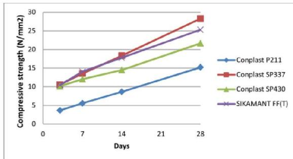
Fig 4. Compressive Strength of Mortar Cube
