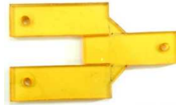
Fig. 12. Photoelastic model of Arc Welded Lap joint Material fringe value F\sigma (Determined using Circular disk) is found out to be 10.242 N/mm.
