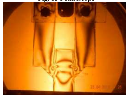
Fig. 14 Isochromatic fring pattern of Lap joint
