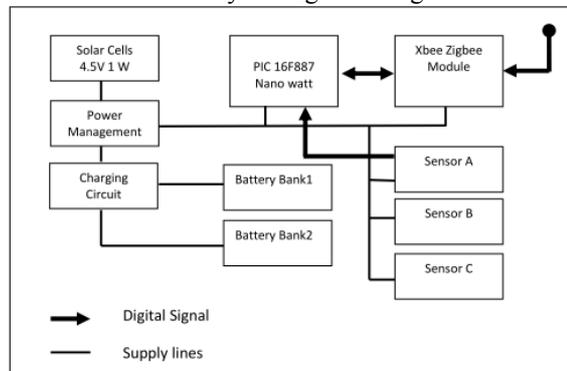
**Figure 3: Architecture of Battery Management Algorithm**
