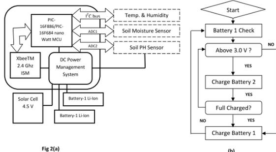
**Figure 2: (a) Sensor node architecture system that features optimal power management system and (b) Battery management algorithm**
