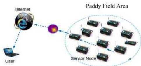
**Figure 1: Wireless Sensor Network routing via PAN both ad-hoc or planned network**
