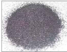
Fig.1.2 Grinded copper slags from industry
