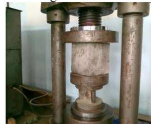
Figure 3.1 Compression Testing Apparatus.
