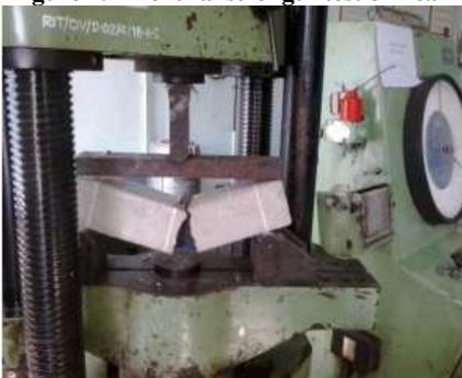
Figure 4.3 Flexural strength test of Beam
