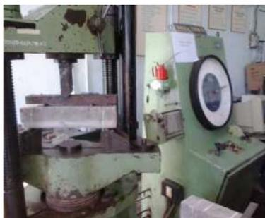
Figure 3.2 Flexural Strength Testing Machine
