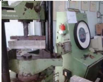
Figure 4.2 Flexural strength test of Beam
