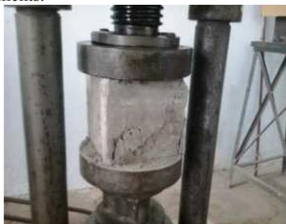
Figure 4.1 Compressive strength test for Cube
