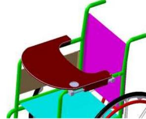
**Fig. 4.5 Three dimensional model of tabletop**
