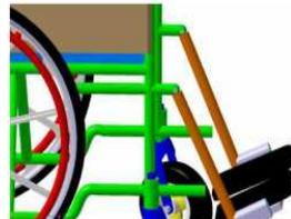
**Fig: 4.4 Three dimensional model of Front Rigging**
