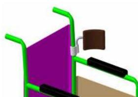
**Fig: 4.3 Three dimensional model of Thoracic support**
