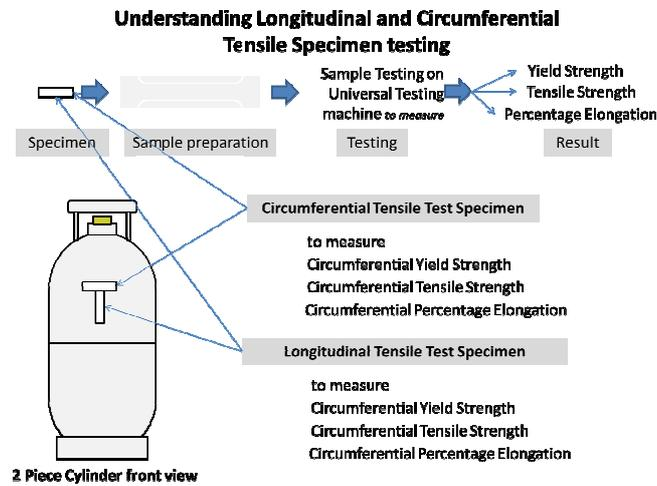
**Fig.2 Acceptance test of LPG Cylinders**
