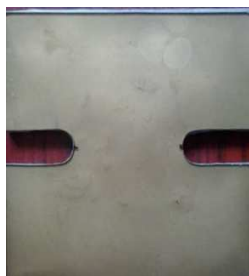
Fig. 01 PhotoStress coated double notched composite panel
