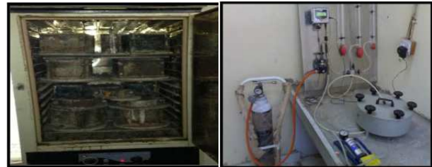
Fig.3 curing of concrete batch at 100°C at oven
