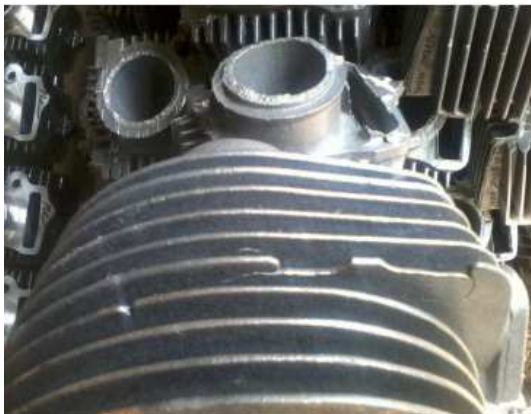
Fig.1 Cold shut in automotive cylinder block
